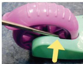
The test examined whether the gap between the wheel and frame could cause fingers to become trapped.
